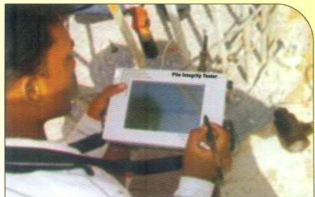
Low Strain Pile Integrity Testing
