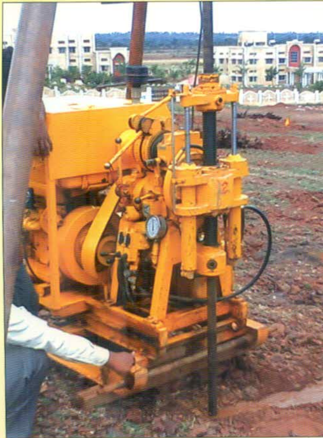
Geo Technical Investigation of Bridge Foundations by Hydraulic Rotary Drilling Machine to Economise Foundations Design
